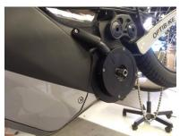
**Step 6:** Loosen the three M6 Allen bolts on motor mount 3 turns. Use 5mm Allen Wrench.
