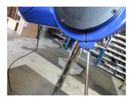
**Step 2:** Slide Motor about 1 inch into frame.
