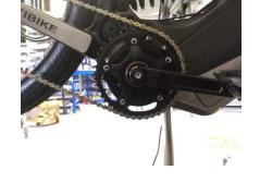
**Step 2:** Remove the 2ea crank arm fixing bolts with 8mm Allen Wrench.
