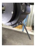
**Step 6:** Install the sprocket, washer and nut. Hold the sprocket with a smooth object inserted through sprocket. Tighten with 1 ¾ inch wrench.
