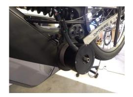
**Step 3:** Connect the motor wires and gently press wires into frame as you slide the motor in.
