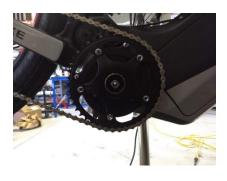
**Step 3:** Remove the crank arms with the crank arm removal tool. (Be sure to screw the tool completely into crank arm before removal)
