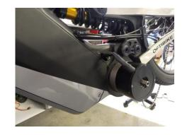
**Step 9:** Pull the connector apart. The small black one has a clip to depress to separate them. The larger motor connector must be pulled apart with force. DO it slowly.
