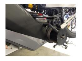
**Step 4:** Press motor into frame until left cover is about 20mm from frame edge. (The motor wire grommet will be touching frame at this distance).
