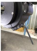
Step 7: Gently Press straight blade screwdriver into gap on motor shell near center bolt to spread motor shell slightly. (Do not over spread shell. Do not twist screwdriver. Press in straight, just enough so motor will begin to slide out.)
