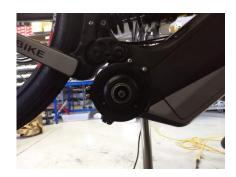
Step 4: Remove the 1 ¾ inch nut from the Sprocket Carrier on right side. Place the 8mm Allen wrench or other smooth object through the sprocket to prevent rotation while removing nut. Turn CCW to remove.
