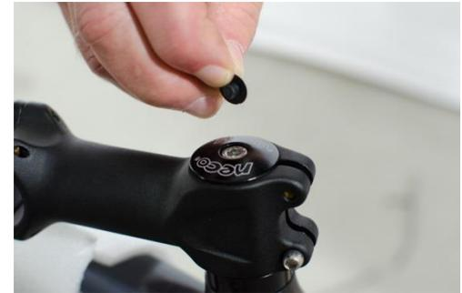
Gently tighten the two stem bolts back and forth until both are evenly tight. (do not tighten one all the way first)
