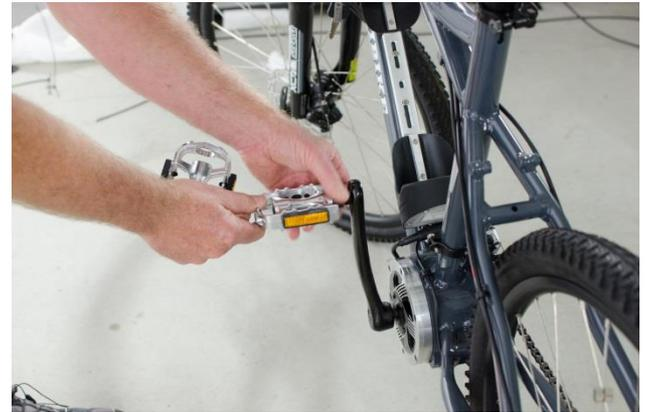
Find the right pedal and verify the “R” mark on the pedal.
