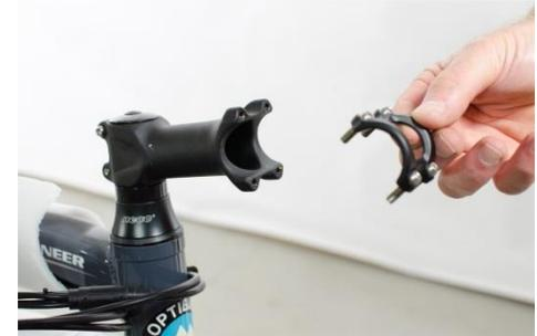
Cut the plastic ties that hold the handlebar to frame.
