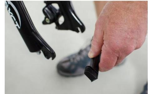
Pick up the bike and insert the axle in the fork. Make sure the disk is aligned between the disk brake pads.
