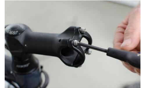
Remove the handlebar clamp
