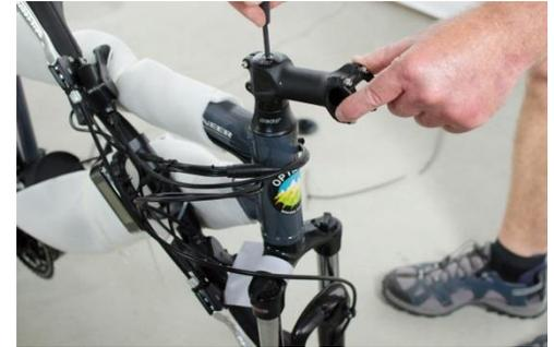
Replace the rubber cap on center Allen bolt.
