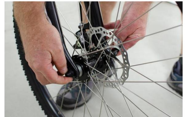
**Caution:** Failure to correctly tighten the front wheel skewer can result in severe injury.
