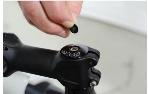
Loosen the bolt 1/2 turn with a 5mm Allen wrench.
