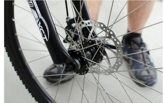
Tighten the nut on right side of wheel skewer a few turns.
