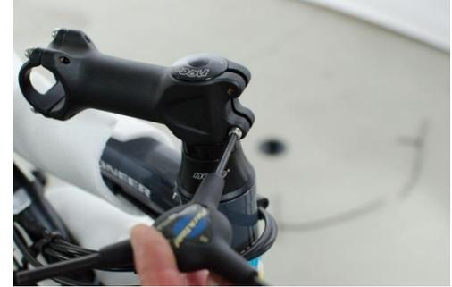
Remove the rubber cap on center Allen bolt.
