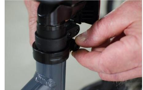
Adjust the seat so it is aligned with frame tube. You can adjust the height of the seat after the bike is assembled.
