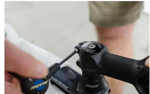
**Caution: Failure to correctly tighten the handlebar stem can result in severe injury.**
