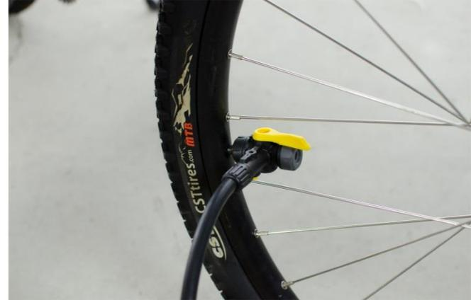
Inflate to about 35 PSI or your desired pressure. Do not exceed the pressure rating listed on the tire.
