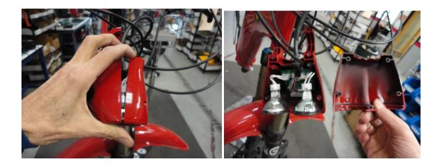
4. Pull off the throttle connector from the display board.
