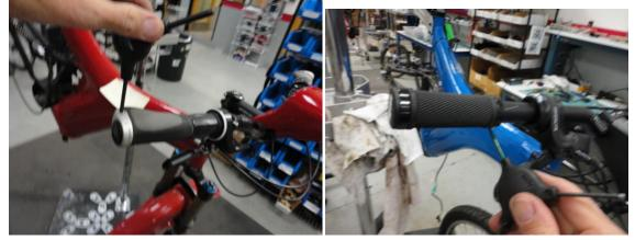
2. Remove headlight bracket clamps using a 2.5mm allen.
