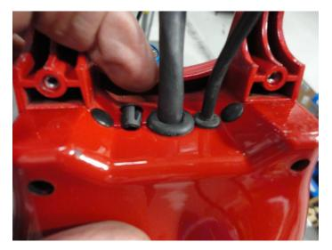
11. Install your headlight body onto the handlebars using a 2.5mm allen. Make sure your cable routing is very similar to the picture and zip tie the throttle cable to the brake line for a clean and secure look.
