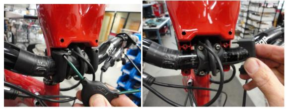
3. Remove bottom of headlight body using a 2.5mm allen. Be careful when you have all 5 screws out as there are 3 caps that could fall out. (see picture)
