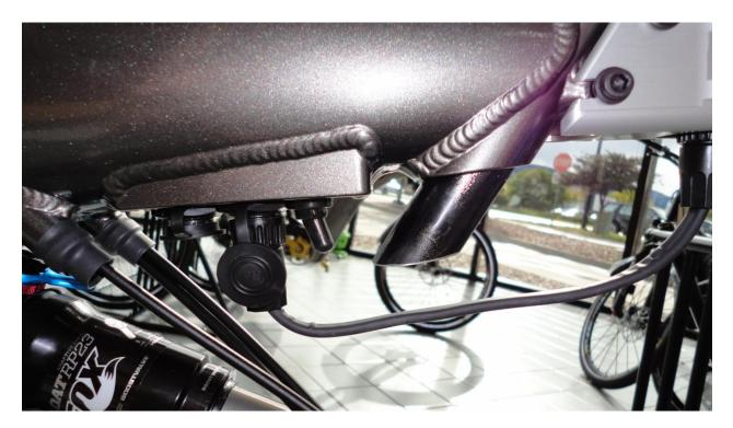
8. To charge your external battery, use the supplied charger (with orange dot) and plug it into the three prong port (rear port) on the external battery as shown in picture below. To charge the external battery the bike does not have to be on. The external battery can also be charged without being connected to the Optibike.
