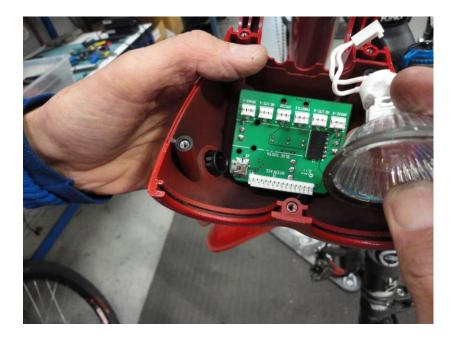
5. Using a 10mm socket or wrench remove the 3 toggle boots that are holding the display board onto the headlight body.
