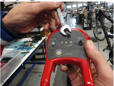
8. Reinstall the headcable, throttle, and headlight bulbs back into the proper connections.
