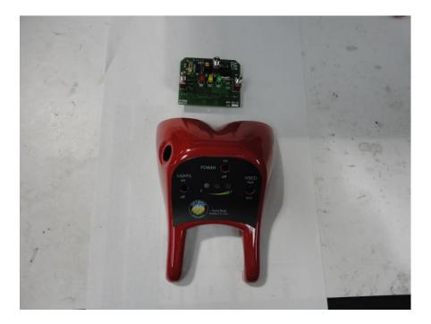
7. Now you can install your new display board, by gently pressing it into the headlight body and tightening the toggle boots back on.
