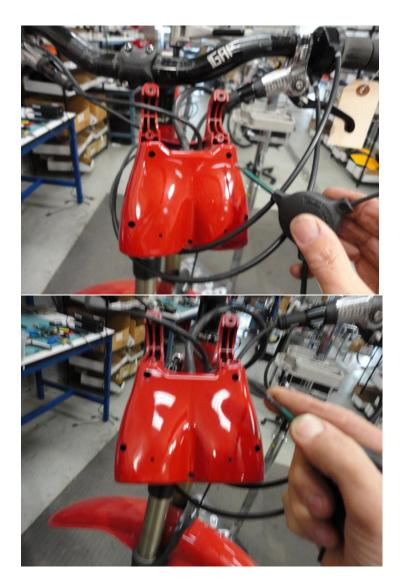
3. Carefully separate the top from the bottom. This will require some force as the headlight bulbs have double sided tape on them to make a seal with the headlight boby.
