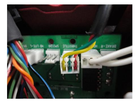
9. At this point you will want to make sure all your cable routing looks fine and align the headcable and throttle grommet as shown. And press and hold the bottom of the headlight body to the top while screwing in the 5 3mm screws.
