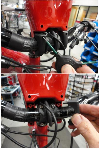
2. Remove the bottom of the display board using the same 3mm allen. There are 5 screws holding it together.
