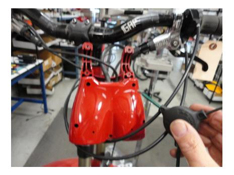
10. Once you have all 5 screws holding the headlight body together press in the 3 plastic plugs as shown.
