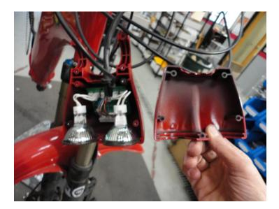
4. Remove all connections from the display board.
