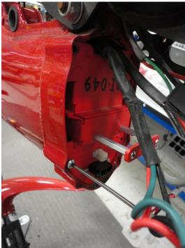
5. Making sure your relay and headlight switches are in the off position. Now you can connect your battery. Orient the wires as shown.
