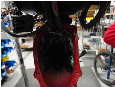
2. Begin to guide battery into frame as shown. While centering wires so the battery support pins do not catch on them.
