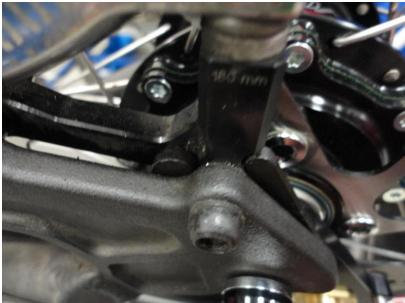
14. Tighten down the quick release. Test to make sure the wheel spins freely.
