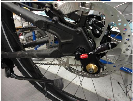
15. Now while in 14 gear attach the rohloff gear box to the transfer arm. Subtle movement of the shifter can help align the two while installing it.
