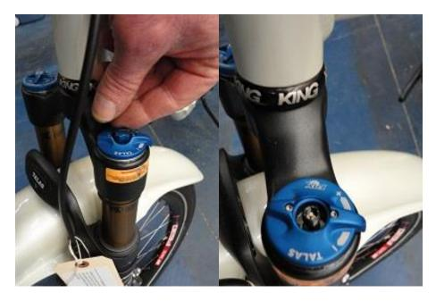
Then thread the shock pump into the fork
