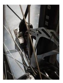
When this is done reinsert the axle, tighten it firmly and press the lock levers into place
