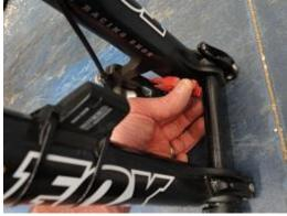
Remove the axle by first flipping down the lock levers (this may vary depending on your model fork/wheel) then unscrewing the axle.
