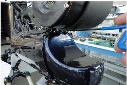
7. Unplug the 8 pin and 3 pin MBB connectors. Using the Molex connector pin removal tool, remove the large 3 pin connector from the pins.
