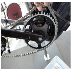
3. Using the 8MM hex wrench remove the crank bolts from the crank arms. Then using the square taper crank puller, remove the crank-arms from the MBB.
